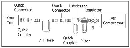
Figure 1. Typical filter/lubricator/regulator installation order.
